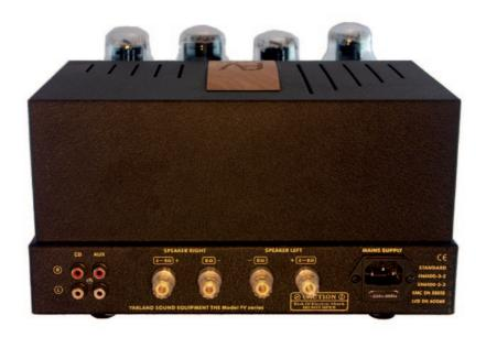
Yarland FV35A: Class A, 2A3 parallel single ended amplifier. The FV35A is quite unusual. A directly heated triode design with two single plate 2A3 tubes per channel. If you find the right speakers to match its low power output, this is your ticket to directly heated triode heaven.
